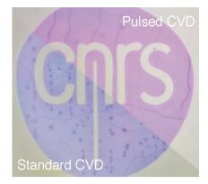
A pulsed chemical vapor deposition (CVD) process for graphene growth on copper foils is introduced. The pulsed injection of carbon precursor efficiently prevents the formation of multilayer patches that is found to affect optical and electronic properties of graphene and leads to homogenous macroscopic graphene sheets.
